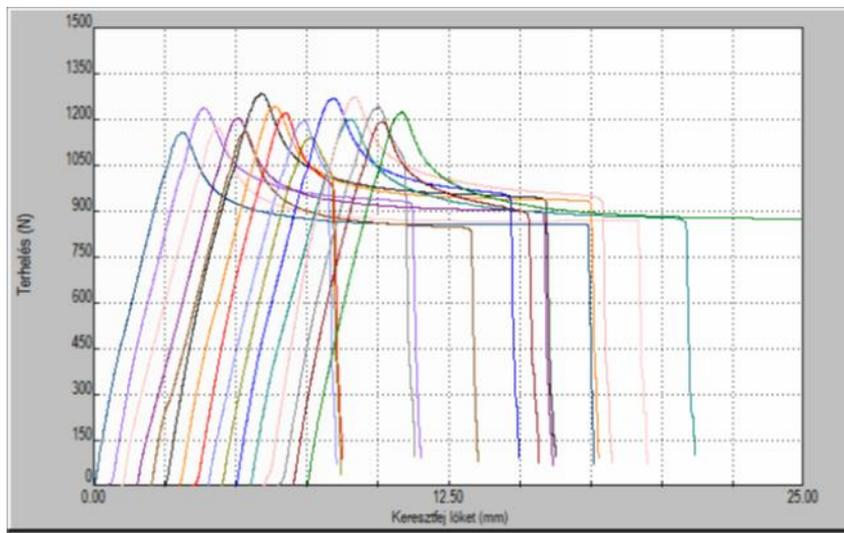
Figure 9 ABS tensile test results
