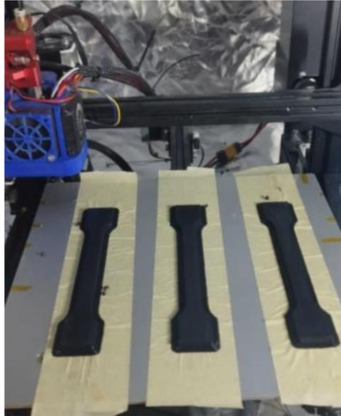
*Figure 3 Printing of ASA tensile test specimens*
