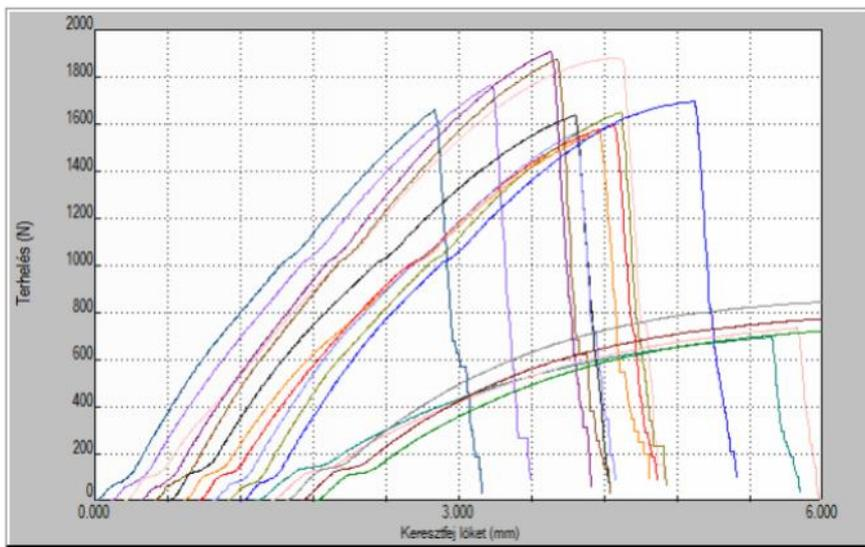
Figure 13 Basic resin tensile test results
