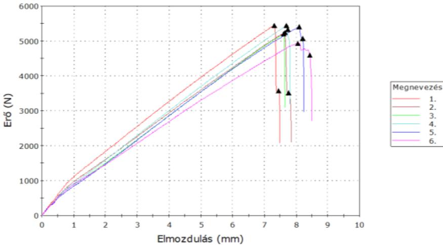
Figure 12 Onyx tensile test results
