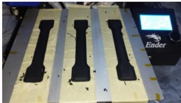
Figure 2 Printing of ABS tensile test specimens ASA
