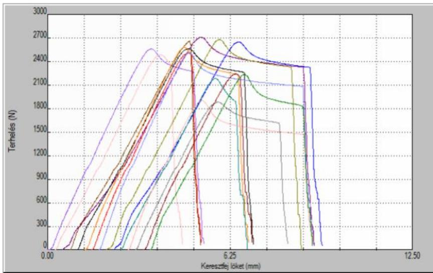
Figure 6 PLA tensile test results
