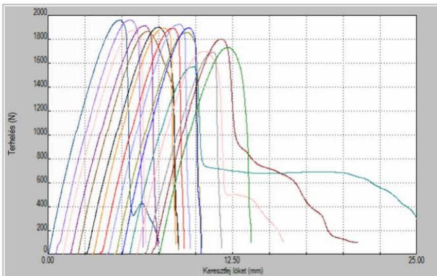
Figure 8 PET G tensile test results
