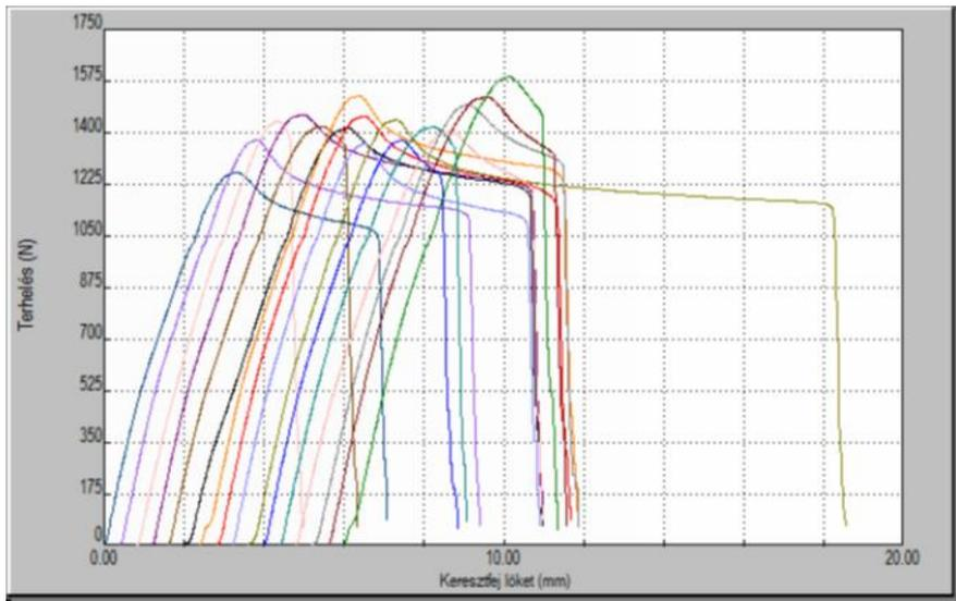
Figure 10 ASA tensile test results
